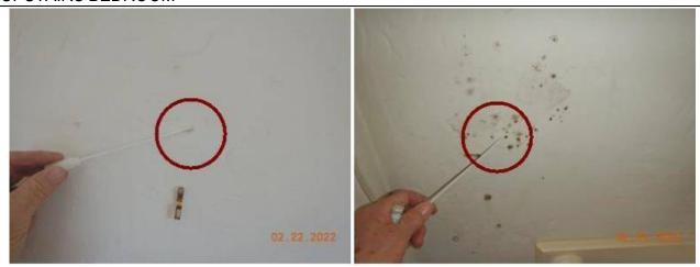
The black smudges on the wall and in the closet proved to not be any type of mold and would not have contributed to the increased level of mold in the air sample.
